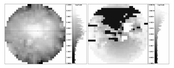
Fig. 3 Resistivity topograms of 2 inch SI SiC wafers [4]. The wafer on the left side is entirely SI in the  $10^7 \Omega$ cm range. The wafer shown on the right side is SI in the  $10^{10} \Omega$ cm range, but a portion (black triangular area) is below  $10^5 \Omega$ cm.
