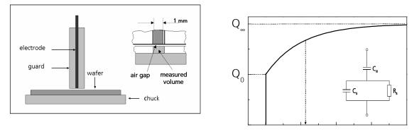
Fig. 1 Left: Schematic representation of the COREMA measurement system. Righ? Charge transient observed after application of a voltage step. The quantities needed to calculate  $\rho$  with eq. (1) are indicated. The insert shows the equivalent circuit of the capacitive probe. The transient time depends on the resistivity and is about 10 µs for  $\rho = 10^7 \Omega$ cm.
