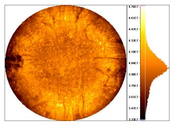
Fig. 2. Resistivity topogram and histogram of a semi-insulating 150 mm Ø LEC grown GaAs wafer.
